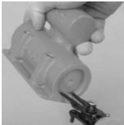
Step 2. Figure 2 With snap ring pliers, remove the bottom end cap retaining snap ring. ( Figure 2 )
