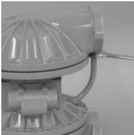
Step 8. Figure 8 To allow for easy removal of the right liquid chamber, first detach the nylon tubing connecting the left air chamber to the right liquid chamber. (Figure 8)
