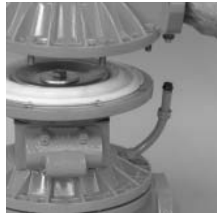
Step 10. Figure 10 Lift liquid chamber away from center section to expose diaphragm, outer piston, and shaft bolt. (Figure 10)
