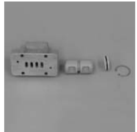
Step 4. Figure 4 Inspect the cylinder end caps, end cap O-rings and piston guide pin. Ensure that guide pin is straight or the piston will not move freely in the cylinder. Inspect the anti-centering pin holes found at the ends of the air valve piston and ensure they are free of debris. Clean filter by removing reducer bushing. Replace air valve gasket if necessary. ( Figure 4 )
