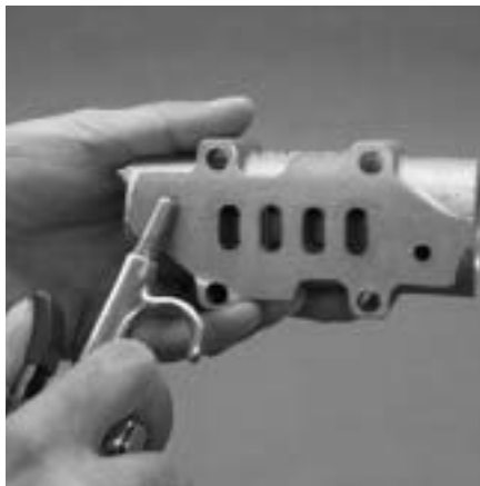
Step 3. Figure 3 Apply pressurized air to the 5 mm ( \frac{1}{8} " ) hole on the opposite end of the air valve face. CAUTION: The air valve end cap may come out with considerable force. Inspect the piston and cylinder bore for nicks and scoring. ( Figure 3 )
