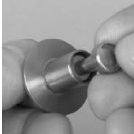
Step 16. Figure 16 Reverse the actuator pin and use it to remove the elastomeric spring. ( Figure 16 )
