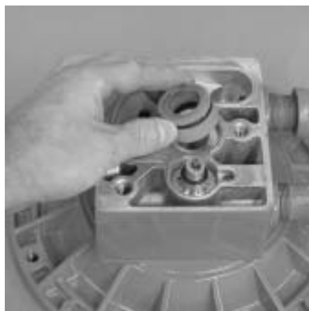
Step 10. Figure 10 Using your thumb, or by pushing on the lip from the opposite side, remove the shaft bushing and replace if necessary. If Glyd™ rings are worn, replace with P/N 08-3210-55-225. ( Figure 10 )
