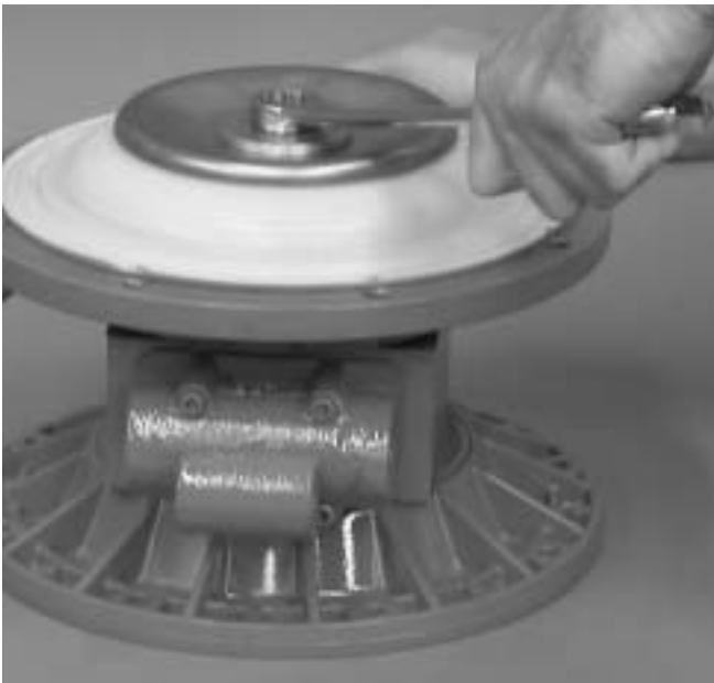
Step 13. Figure 13 Using a 19 mm ( \frac{3}{4} " ) wrench, remove the left shaft bolt by turning counter clockwise. ( Figure 13 )
