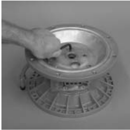
Step 6. Figure 6 Remove the air chamber bolts with a 6 mm (¼") hex head wrench. ( Figure 6 )
