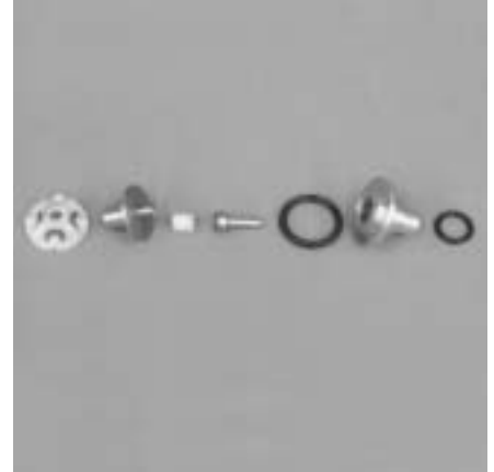
Step 17. Figure 17 The pressure relief assembly is comprised of 7 distinct parts ( Figure 17 ). An entire pressure relief valve assembly can be purchased or a seal kit can be purchased to rebuild the entire pressure relief valve. IMPORTANT: Both sides of the pump must be rebuilt at the same time.
