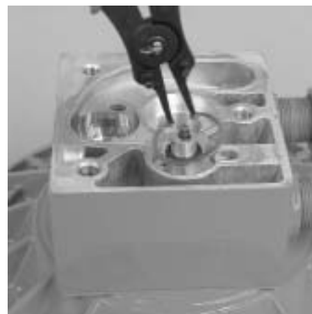
Step 11. Figure 11 Using snap ring pliers, remove the snap ring pressure relief retainer. ( Figure 11 )
