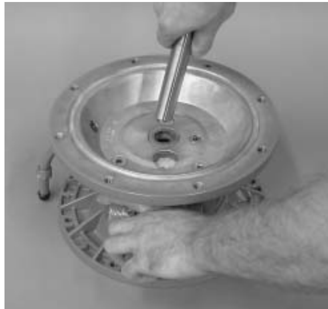
Step 14. Figure 14 Now that both diaphragm assemblies have been removed from pump, remove main shaft from center section. ( Figure 14 )
