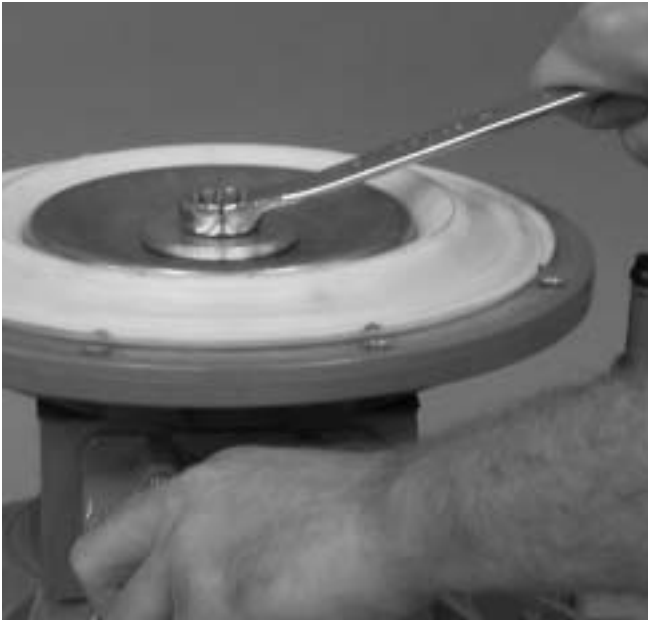
Step 11. Figure 11 Using a 19 mm ( \frac{3}{4} " ) wrench, remove the shaft bolt by turning counter clockwise. ( Figure 11 )
