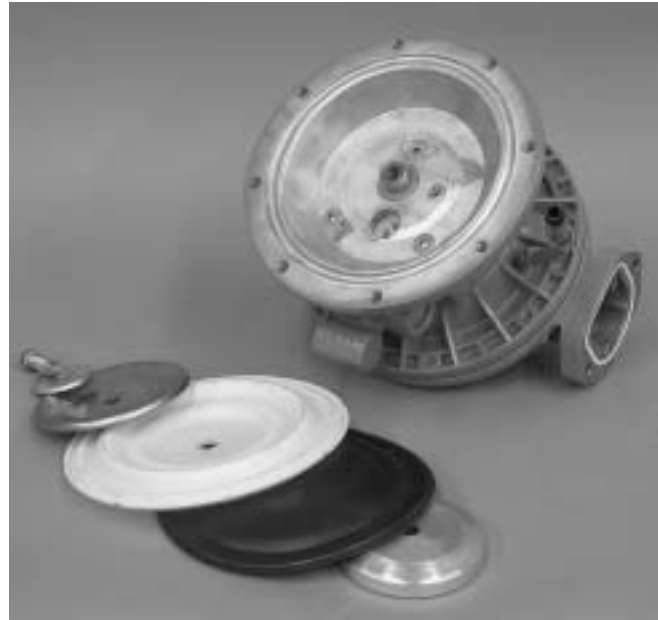
Step 12. Figure 12 After removing the shaft bolt, outer piston, and diaphragm from right side of pump, remove left liquid chamber. ( Figure 12 )
