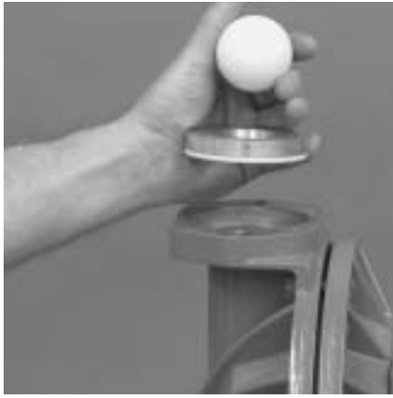
Step 5. Figure 5 Remove the discharge valve ball, valve seat, and valve seat O-ring from the left liquid chamber and inspect for nicks, gouges, chemical attack or abrasive wear. Replace worn parts with genuine Wilden parts for reliable performance. The Teflon® valve seat O-rings should be replaced when pump is reassembled. (Figure 5)
