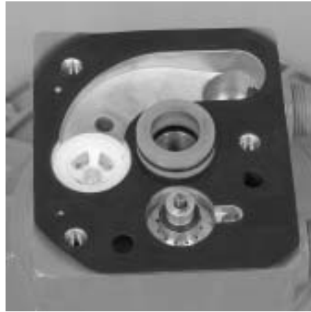
Step 7. Figure 7 Remove the air chamber gasket. Inspect gasket for signs of wear or chemical attack and replace if necessary. ( Figure 7 )
