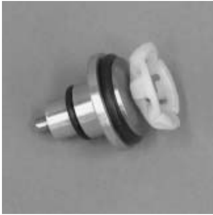
Step 12. Figure 12 The entire relief assembly can be removed from the center block ( Figure 12 ). Notice that the legs of the elastomeric spring point away from the assembly.
