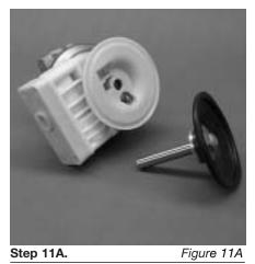
NOTE: Due to varying torque values, one of the following two situations may occur: 1) The outer piston, diaphragm and inner piston remain attached to the shaft and the entire assembly can be removed from the center section. (Figure 11A)
