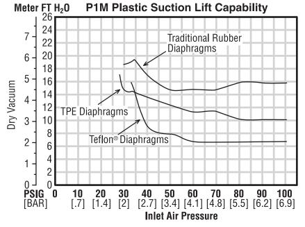
These vacuum numbers will double when a small amount of back pressure is placed on the discharge.
