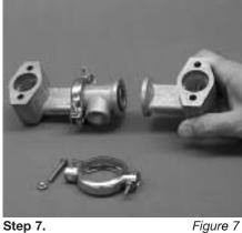
Inspect O-rings for wear or damage and replace if necessary. Teflon® O-rings should be replaced when reassembled. (Figure 7)
