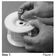
Remove pilot spool sleeve from center section (Figure 7).
