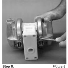
Use a 3/6" wrench to remove one set of clamp bands that secure one liquid chamber to the one-piece center section. (Figure 8)
