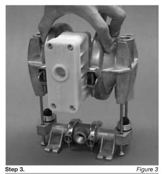
Remove the top manifold and lift the center section off the inlet manifold. (*Figure 3*)
