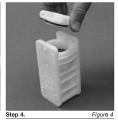
Remove air valve end cap to expose air valve spool by simply lifting up on end cap once air valve bolts are removed. (Figure 4)
