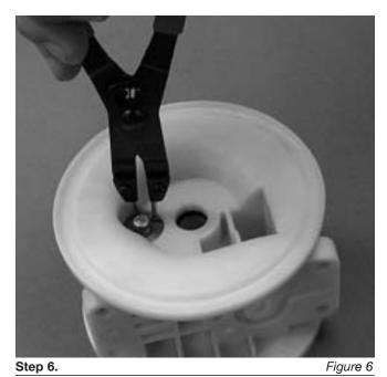
Remove pilot spool retaining snap ring on both sides of center section with snap ring pliers (Figure 6).
