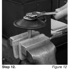
To remove the diaphragm assembly from the shaft, secure shaft with soft jaws (a vise fitted with plywood or other suitable material) to ensure shaft is not nicked, scratched, or gouged. Using an adjustable wrench, remove diaphragm assembly from shaft. Inspect all parts for wear and replace with genuine Wilden parts if necessary. (Figure 12)
