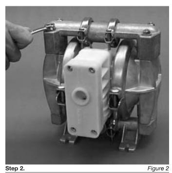
Utilizing the %" box wrench, start by removing the four long carriage bolts that hold the top and bottom manifolds to the center section. (*Figure 2*)
