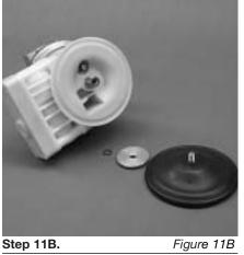
2) The outer piston, diaphragm, inner piston, and disc spring separate from the shaft which remains connected to the opposite side diaphragm assembly (Figure 11B). Teflon®-fitted pumps come standard with back-up diaphragms (not shown).
