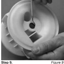
Check center section Glyd<sup>™</sup> rings for signs of wear. If necessary, remove Glyd™ rings with O-ring pick and replace. (Figure 9)
