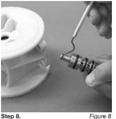
With o-ring pick, gently remove the o-ring from the opposite side of the "center hole" cut on the spool. Gently remove the pilot spool from sleeve and inspect for nicks or gouges and other signs of wear. Replace pilot sleeve assembly or outer sleeve o-rings if necessary. During reassembly never insert the pilot spool into the sleeve with the "center cut" side first, this end incorporates the urethane o-ring and will be damaged as it slides over the ports cut in the sleeve.
