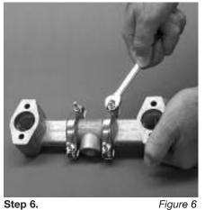
Normally the inlet and discharge manifold should not be disassembled during regular pump maintenance. Should this be necessary, completely remove and disassemble manifold clamp bands utilizing a 7/6" wrench. (Figure 6)
