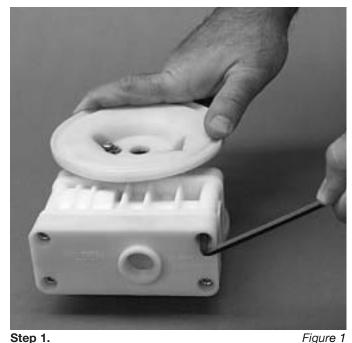
Loosen the air valve bolts utilizing a 3/6" hex head wrench. (Figure 1)
