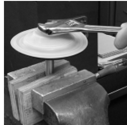
Step 12. Figure 12 To remove the diaphragm assembly from the shaft, secure shaft with soft jaws (a vise fitted with plywood or other suitable material) to ensure shaft is not nicked, scratched, or gouged. Using an adjustable wrench, remove diaphragm assembly from shaft. Inspect all parts for wear and replace with genuine Wilden parts if necessary. (Figure 12)
