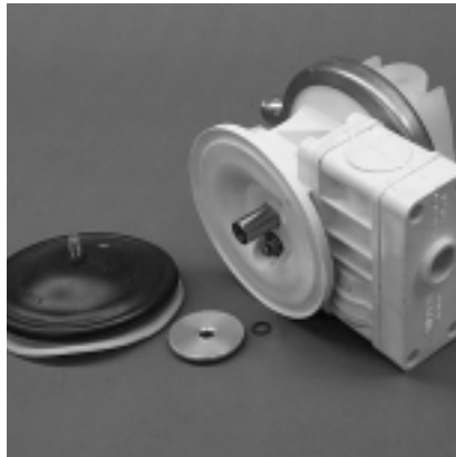
Step 11A. Figure 11A NOTE: Due to varying torque values, one of the following two situations may occur: 1) The outer piston, diaphragm and inner piston remain attached to the shaft and the entire assembly can be removed from the center section. (Figure 11A)
