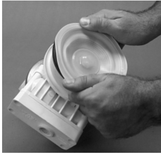
Step 10. Figure 10 Using an adjustable wrench, or by rotating the diaphragm by hand, remove the diaphragm assembly from the center section. (Figure 10)
