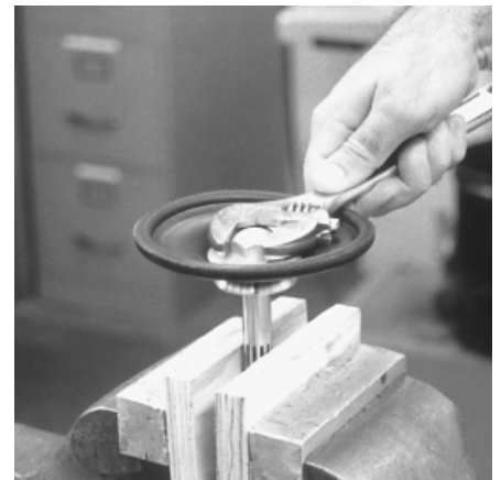
Step 12. Figure 12 To remove the diaphragm assembly from the shaft, secure shaft with soft jaws (a vise fitted with plywood or other suitable material) to ensure shaft is not nicked, scratched, or gouged. Using an adjustable wrench, remove diaphragm assembly from shaft. Inspect all parts for wear and replace with genuine Wilden parts if necessary. ( Figure 12 )
