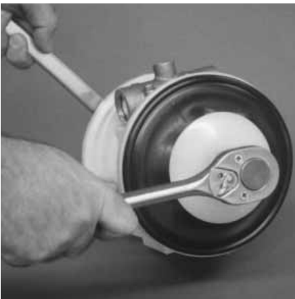
Step 11. Figure 11 Using two 1" sockets, remove diaphragm assembly from center section assembly.
