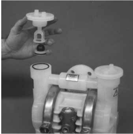
Step 3. Figure 3 Remove the top liquid retainer to expose the valve balls, valve seats and valve seat o-rings.
